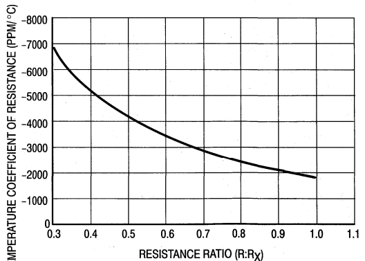
Figure 8. Temperature Coefficient of Resistance for a Series Resistance Required for "Ideal" Span Temperature Compensation versus Resistance Ratio (R:Rx)
